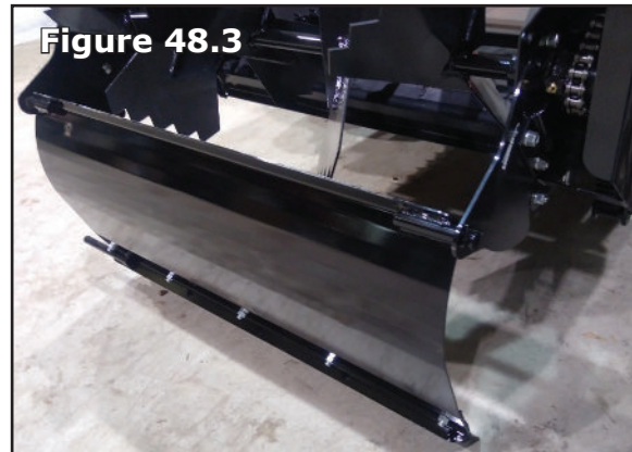
SAFETY BAR REMOVE COTTER PIN ON BOTH ENDS OF SAFETY BAR
